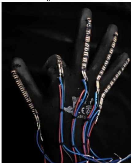
Fig. 4: Sensor state '01000' mapping the letter 'HI'
